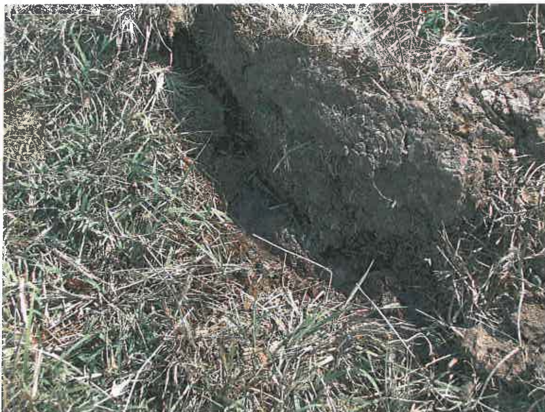
Figure 17: Cross section of soil at top of paddock. Collected water shows impermeability of the soil.
