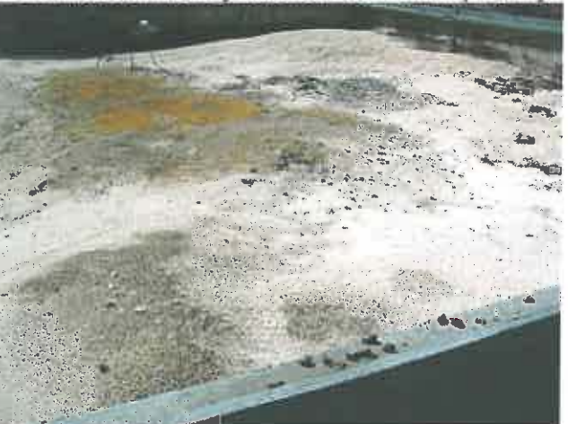
Photo. 3: Sand media of the Hybractor Technology Biofilter showing patches of the "Flowers-of-Sulphur" effect sublimed on the surface. The media box was recently upgraded and painted.
