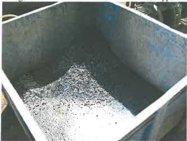
Photo. 8: Balls of fat deposited around keratin cores removed from the primary effluent stream to the Hybractor Primary Digester, using a Trommel Screen Unit.
