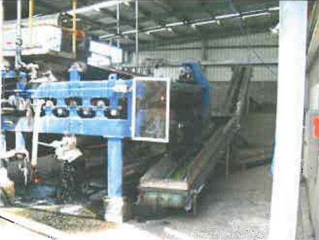
Photo. 16: Hybractor Primary Digester belt press sludge being stockpiled under cover, prior to being included in on-site composting operations. Only minor, local fugitive odour is associated with this material.
