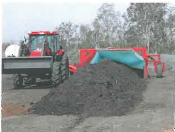
Fig 20: The new windrow turner has a number of plasticised canvas sheets that effectively reduce the amount of dust released by this operation.
