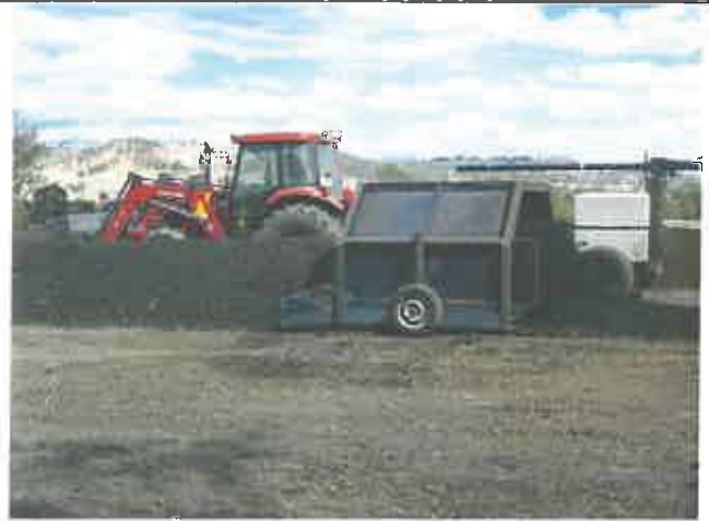
Photo. 24: Commencement of a compost windrow mixing "run". The "swing arm" mounted at the rear of the compost mixing unit (centre, right) can be positioned to place and remove covers from the windrows prior to mixing/aeration (Photos. 17, 23).
