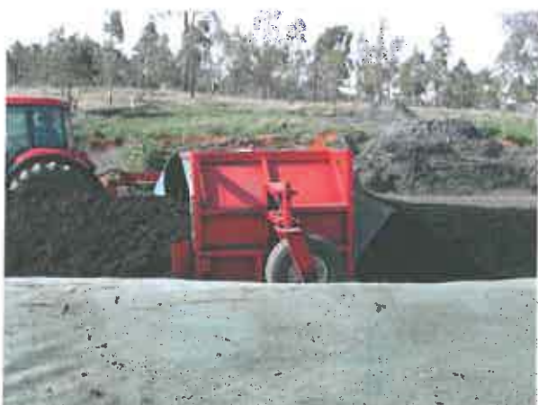
Fig 21: Shows the effectiveness of the windrow turner – before and after compost texture.
