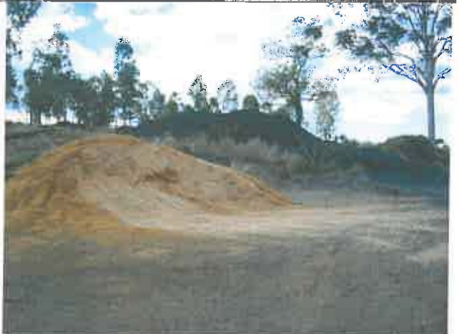
Photo. 19: Compost manufacturing dry raw materials storage area showing sawdust, fly ash, paper ash stockpiles. Any runoff from this area is also directed to the swale system indicated in Photograph 18.
