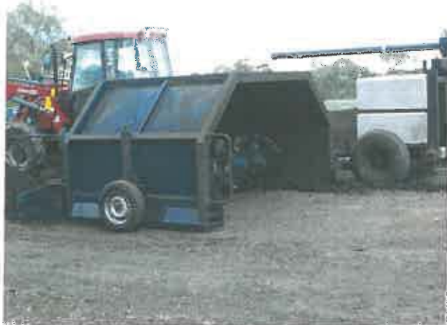
Photo. 23: New compost mixing unit and dedicated "slow-crawl" geared tractor recently acquired by GELITA.
