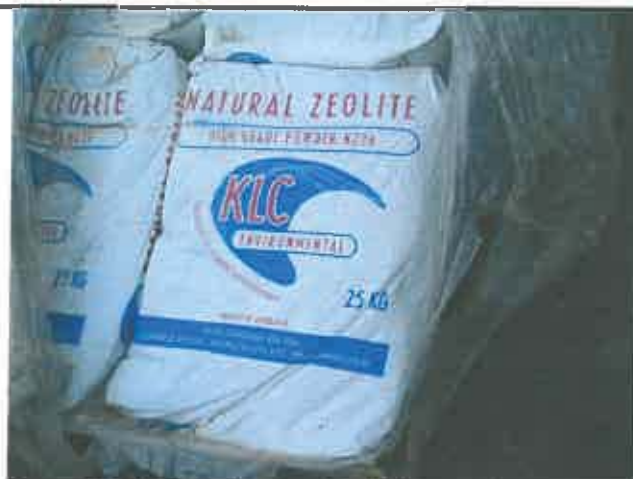
Photo. 14: GELITA is currently trialling zeolite in the Aerobic Pond to determine if the material will reduce the ammonia content of the effluent. Zeolite is also claimed to assist in odour suppression, reduction of chloride levels and the binding of nitrogen.
