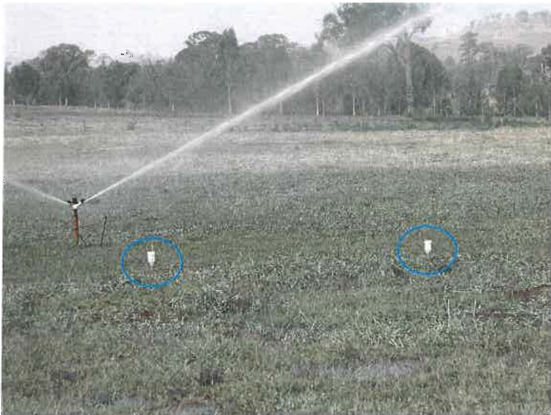
Figure 14: Irrigation system in use. Also visible are access tubes for the neutron moisture meters. (marked) Used to measure effectiveness of irrigation on this particular paddock.
