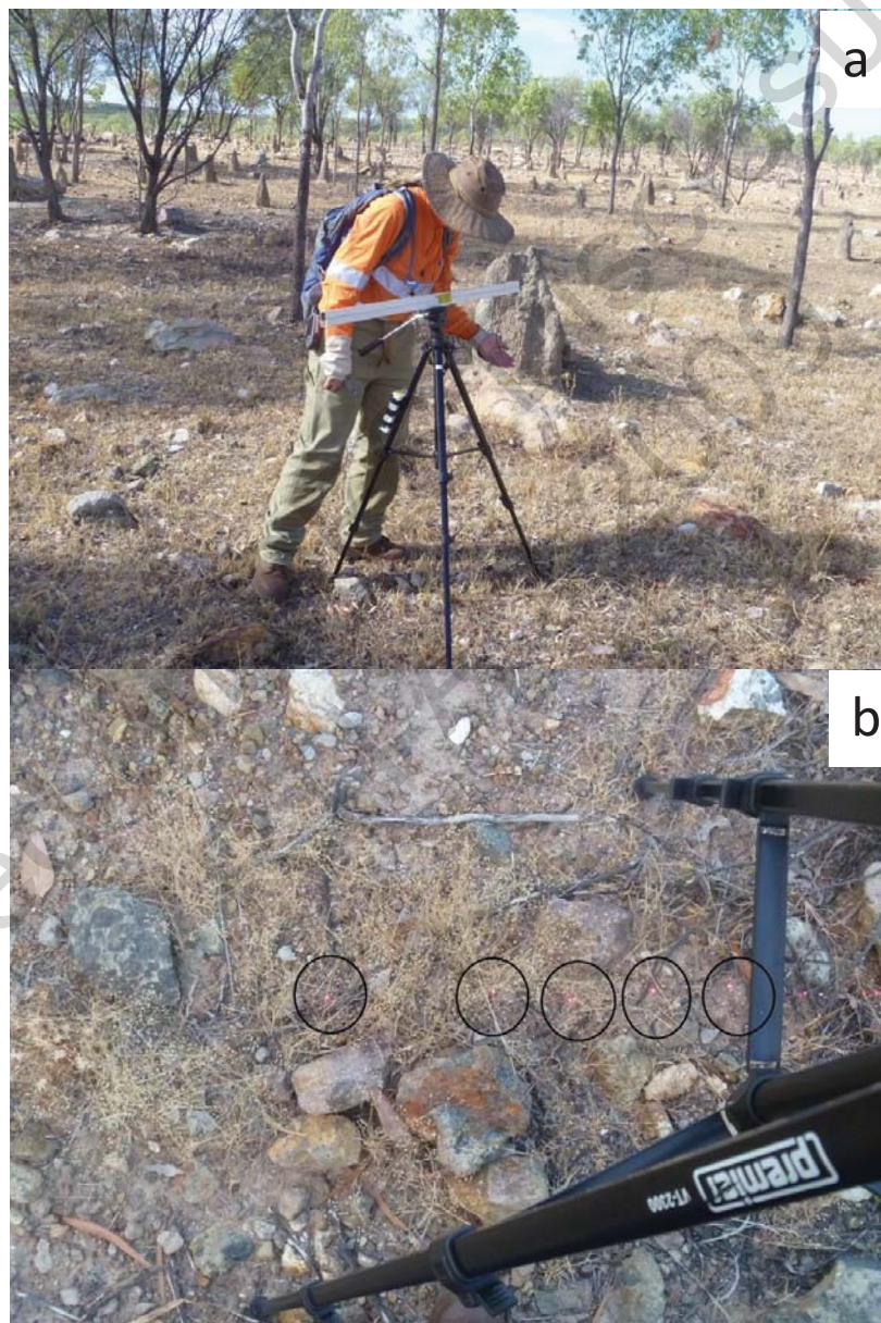
Figure 2. The laser method of sampling the point cover abundance of plants and bare ground etc (developed by Cedar Creek Associates, Colorado USA). The laser dots are circled in photo “b”.
