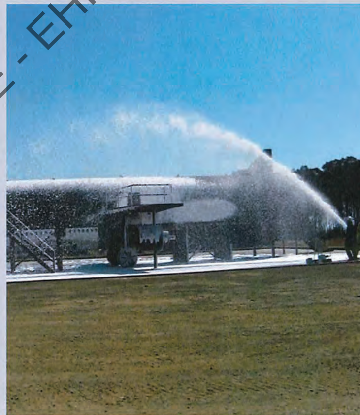
Image: Example of AFFF in use
