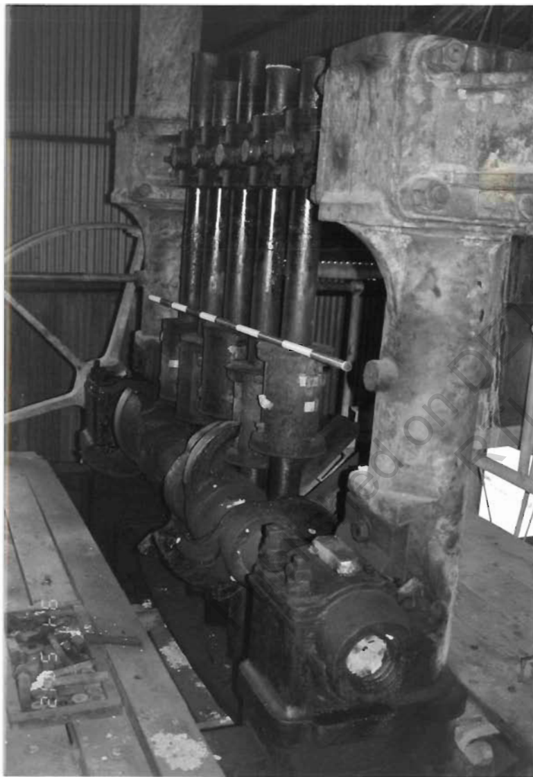
Thompson & Co. stamp battery cam shaft and rods.
