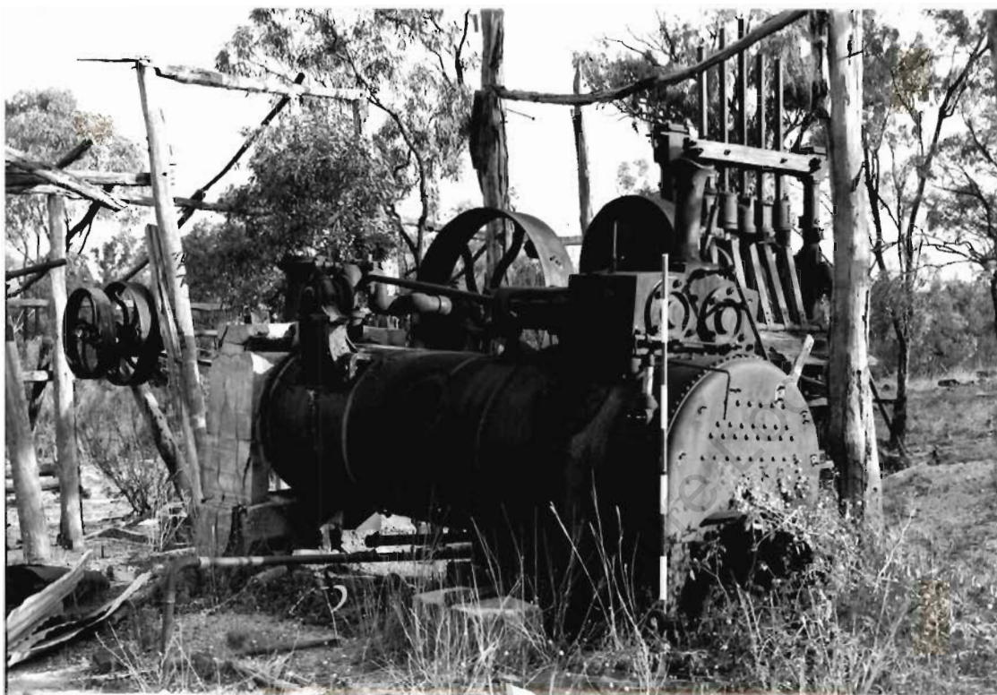
Brown & May 2 cylinder portable engine, looking S.
