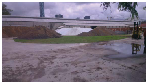
Photo 4 – Surplus stockpiling of crushed glass and silica sand.
