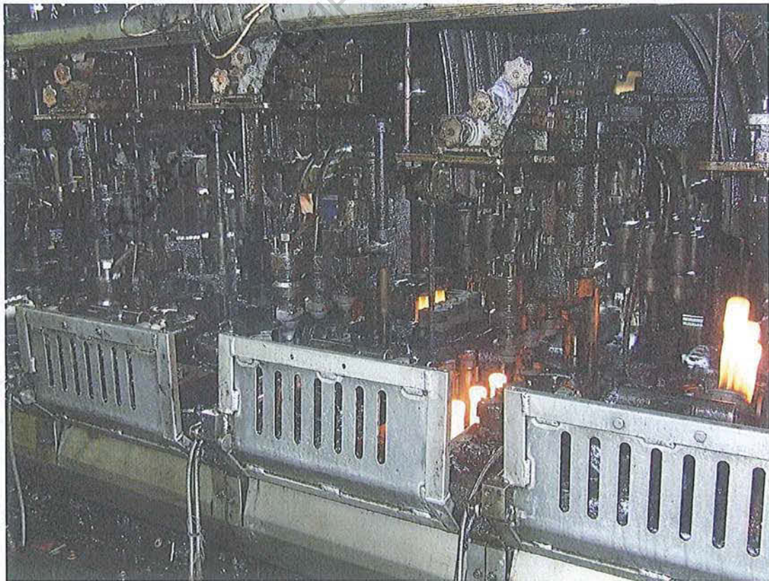
View showing red-hot formed bottles.
