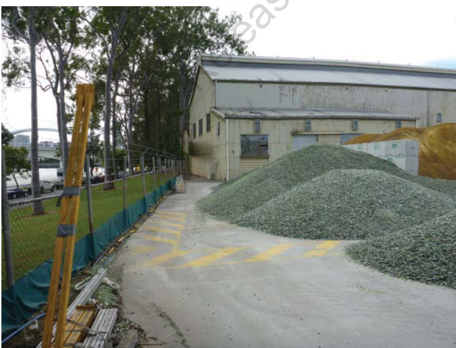
Photo 15 – Glass stockpiles the hardstand. Dust/glass particulate fence along site boundary.
