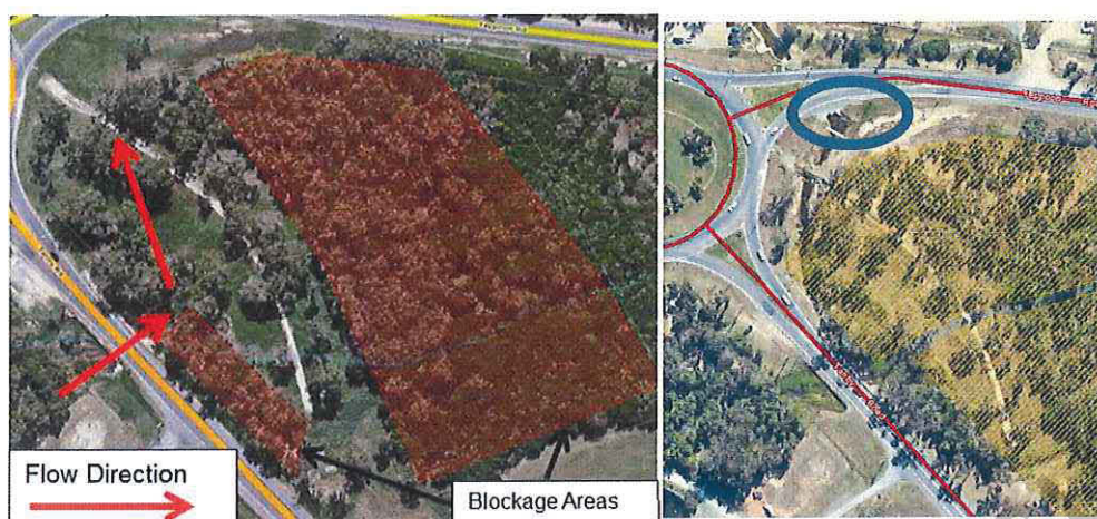
Figure 2 – The image to the left supplied by council shows the Tanby Road culvert flow direction, the image to the right shows the Yeppoon Road culvert (blue circle).
