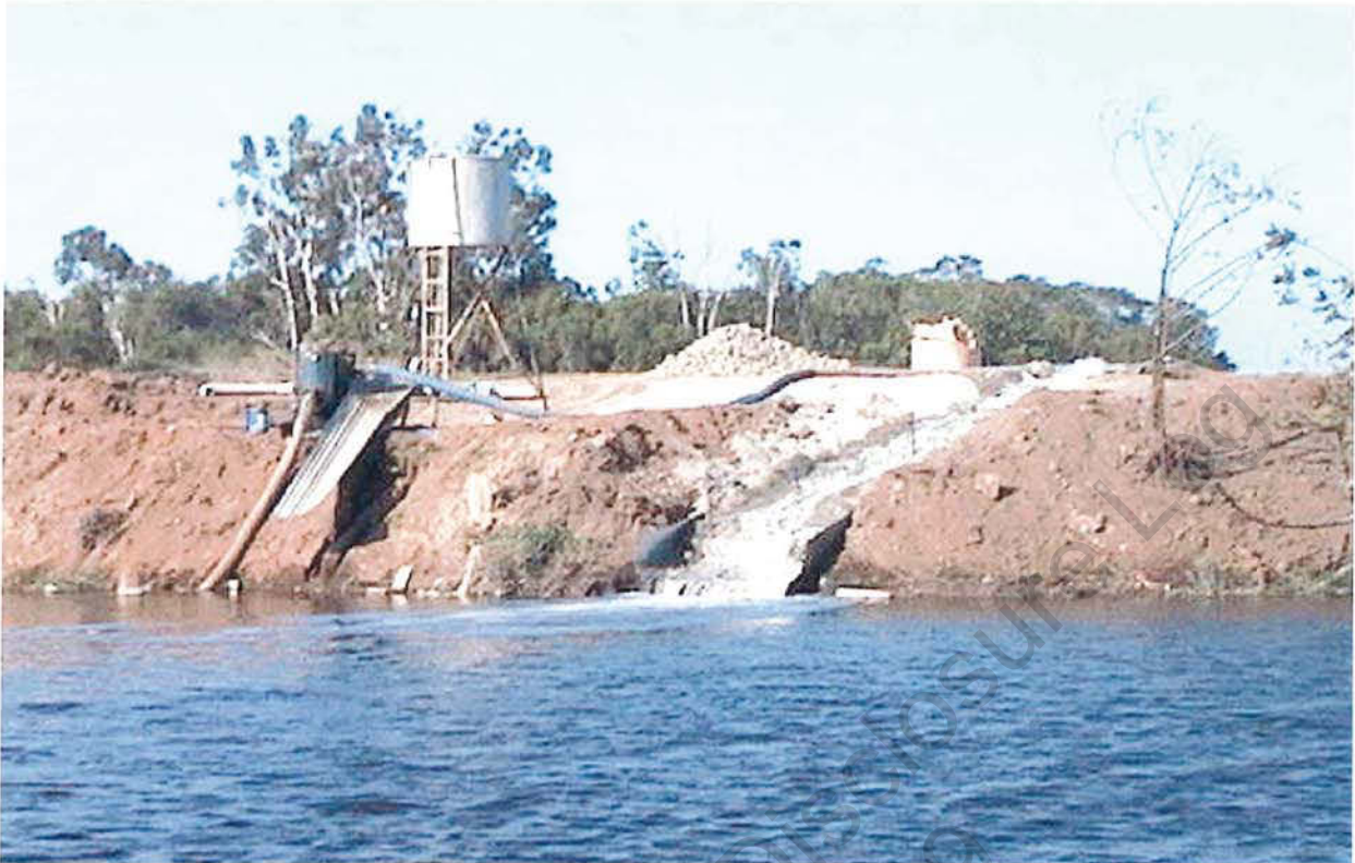
Plate 1 – Illustration showing the artificial waterfall being used to aerate pit waters.
