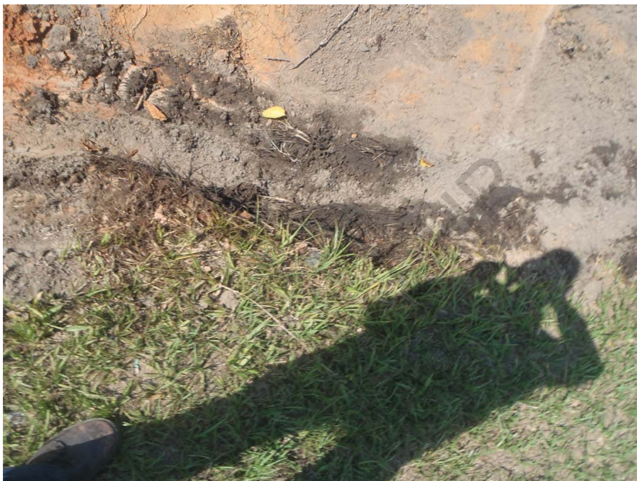
Photo 15 - This photo is taken approximately 30m from the location in photo 14. It shows some contaminated land that remains in the grass spoon drain after the MBRC remediation works.
