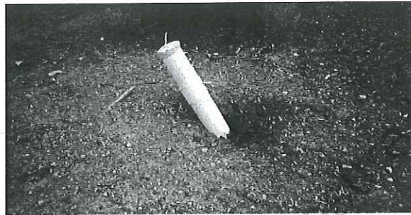
Figure 8 Typical exploration drillhole with PVC collar pipe - note conical concrete plug in top
