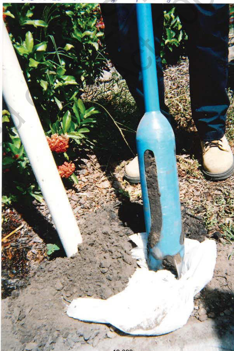
Photo 12: 2/2/06 TP006 Visual staining & strong hydrocarbon odors 1-1.3m depth.
