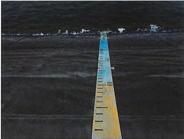
DSCN7794. MRL marker and Brine Pond level marker
