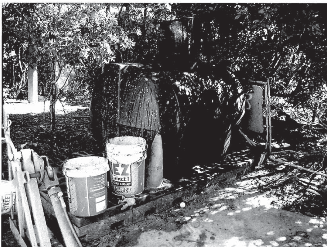
Photo 9 – Emoleum tank situated on a bunded pallet to the north of the main wash bay. The bunded pallet was full of stormwater. The open buckets were also contained an unidentified substance.
