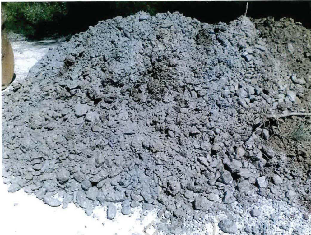
Photograph 6: View of fill material encountered during the excavation of Test Pit 2 (TP2)
