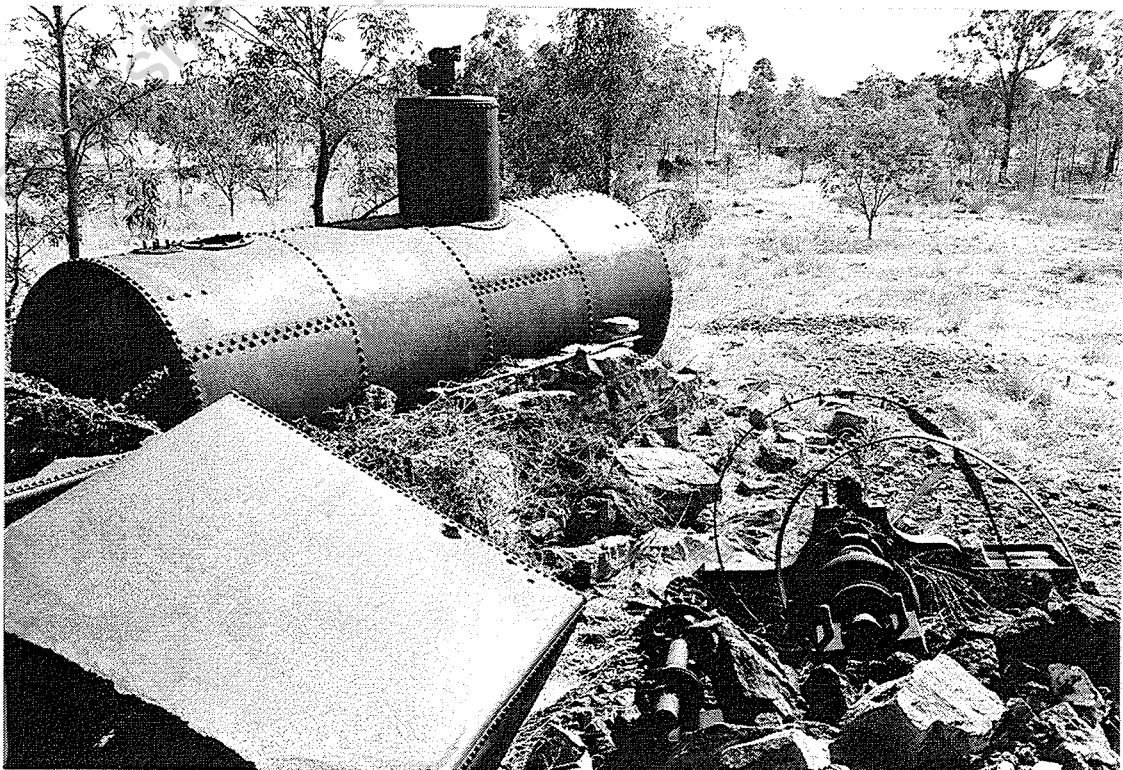
Roger's No.1 mine site showing Cornish boiler with bulldozed winding engine and ships tank.
