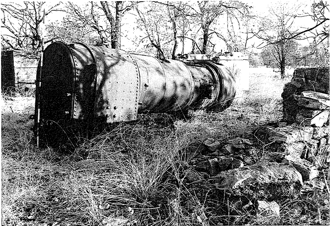
Portable engine with winding engine mounts behind and Cornish boiler mount on left. Looking S.
