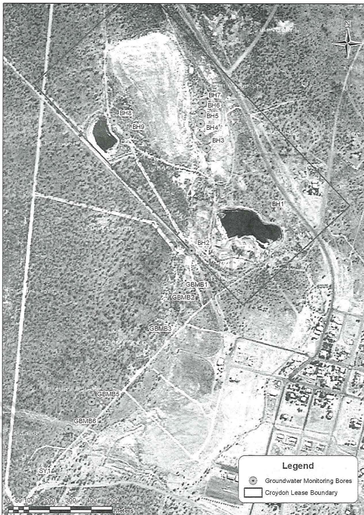
Figure 16: Croydon Groundwater Monitoring Boreholes– South-Eastern Close-up
