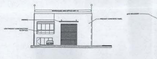
4 WEST ELEVATION UNIT 12 1:300
