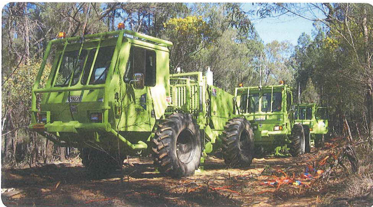
Vibroseis trucks send acoustic waves into the earth. A recording truck is connected to up to 10km of cable to receive the seismic signal.
