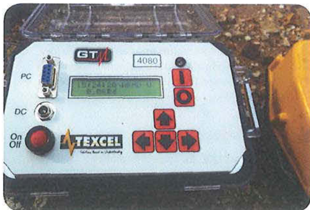
Peak particle velocity meters provide real-time monitoring of vibrations when data is being collected close to sensitive receptors, such as residences.
