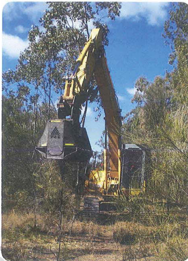
A mulcher used to cut vegetation without damaging root systems.
