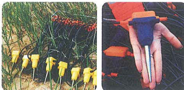
Geophones – sensors are placed along the seismic line.
