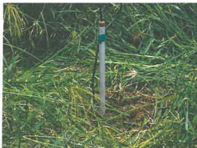
Longstop equipment used for extraction of soil solution for nitrate and salt status below the root zone.
