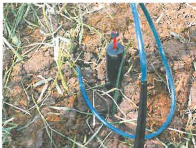
Full Stop Moisture monitoring equipment showing red button up when soil water profile is full at 50 cm
