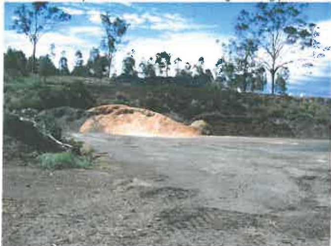
Photograph 9 – Composting raw materials bulk storage area adjacent to the sealed compost mixing/maturing pad, which includes; sawdust, paper-ash, belt-press sludge and mulched green waste stockpiles.
