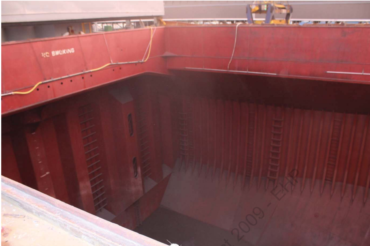
IMG1193 – 19 February 2015, lead dross dust in suspension and leaving hold after spray bars have been turned off.
