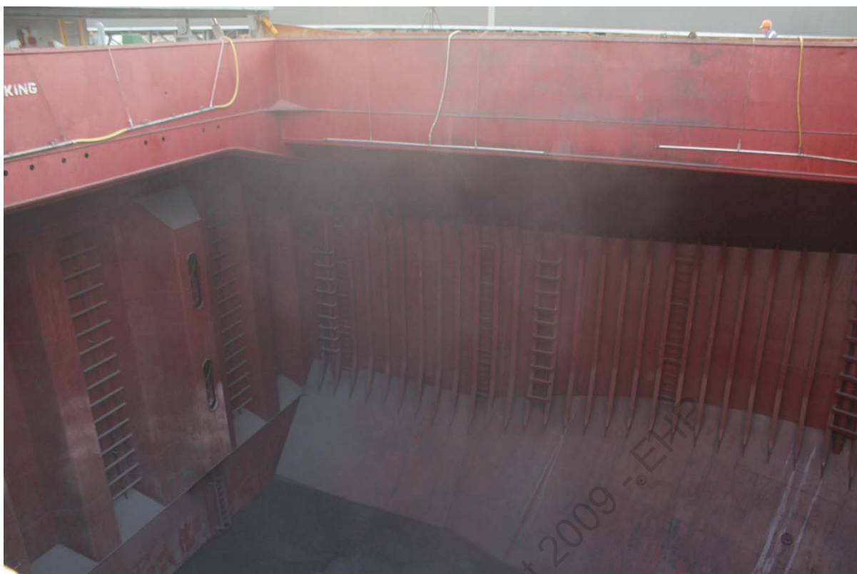
IMG1144 – 19 February 2015, dross dust in suspension after spray bars have been turned off.
