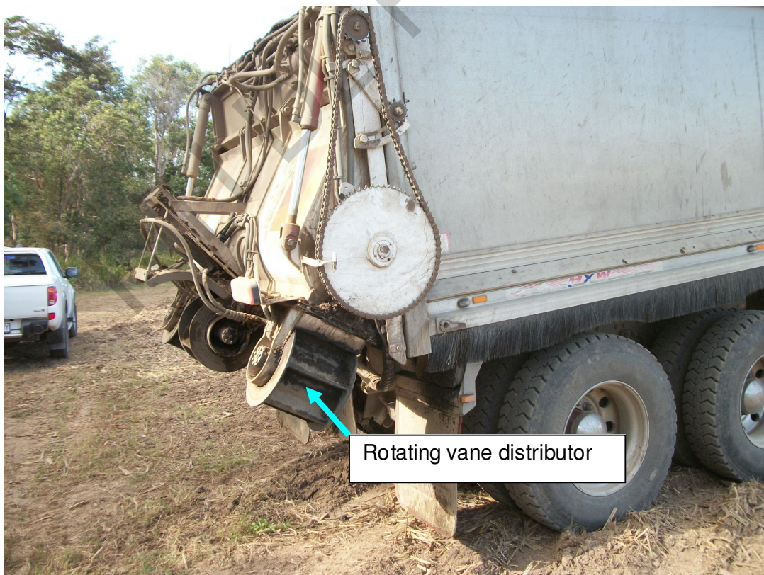
Photo 3 – rotating vane distributor with the tail gate in the distribution position
